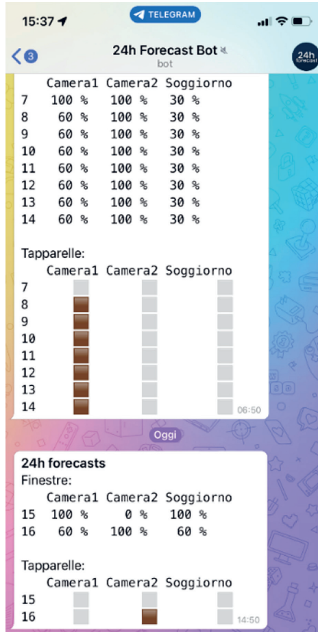
Fig. 2: Sample print-screen of the 24-hour forecasting PREDYCE Telegram bot for the Turin apartment.
