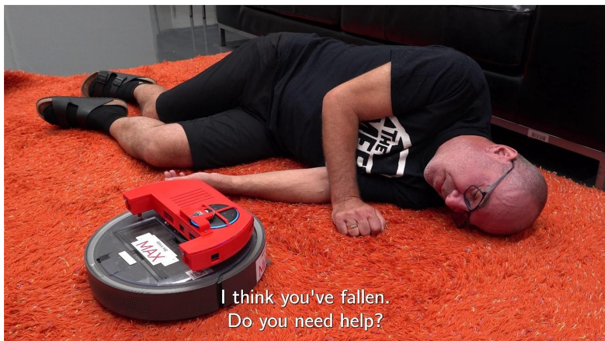
Figure 1 The Smart Companion prototype detected a person on the ground, assumes an emergency and tries to get in touch prior to alerting the emergency assistance.
