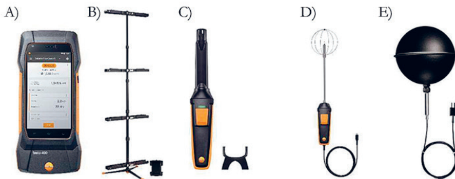
Fig. 1: Measuring equipment for climate-related parameters A) Testo 400 - Universal Air Flow and IAQ Instrument, B) Measuring tripod, C) Testo CO 2 probe including temperature and humidity sensor, D) Testo Turbulence probe, E) Testo Globe Probe
