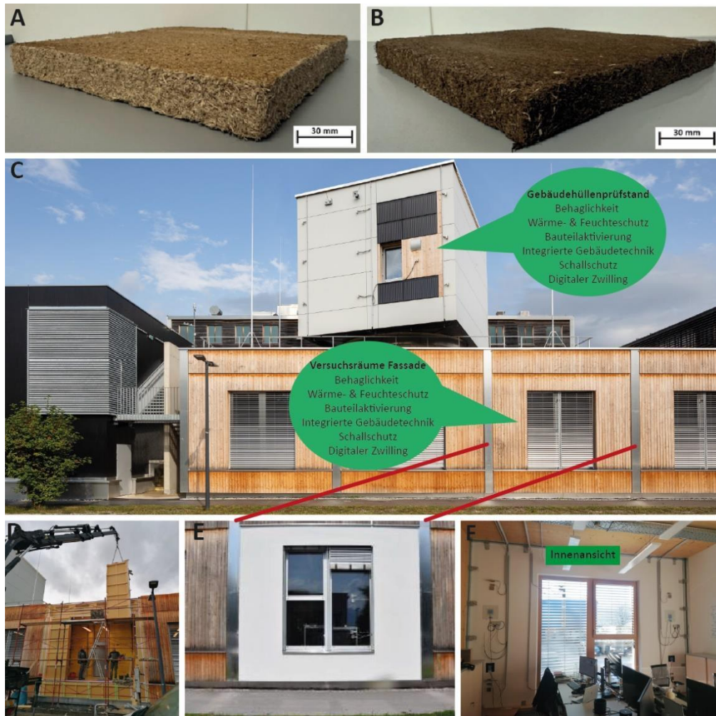
Figure 1 Comparison of WFIB manufactured in the wet process using fresh fiber (A) and composted fibers (B) both bound with 1% cellulose. Outer view of the Twin 2 Sim testing building (C) and: installment (D), outer view (E), and inner view (F) of the demo wall.
